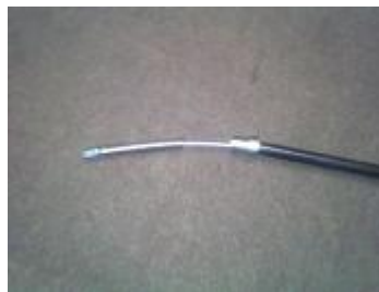
Cable mechanic wires used in automotive – hand brake wires Bowdens with steel wire and special endings
